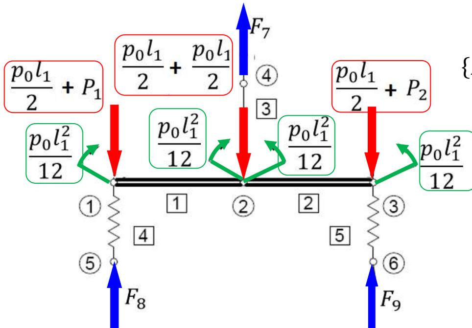
$$\{F\}_g = \begin{Bmatrix} -\frac{p_0 l_1}{2} - P_1 \\ \frac{p_0 l_1^2}{12} \\ -\frac{p_0 l_1}{2} - \frac{p_0 l_1}{2} \\ \frac{p_0 l_1^2}{12} - \frac{p_0 l_1^2}{12} \\ -\frac{p_0 l_1}{2} - P_2 \\ \frac{p_0 l_1^2}{12} \\ F_7 \\ F_8 \\ F_9 \end{Bmatrix} = \begin{Bmatrix} -\frac{p_0 l_1}{2} - P_1 \\ -\frac{p_0 l_1^2}{12} \\ -p_0 l_1 \\ 0 \\ -\frac{p_0 l_1}{2} - P_2 \\ \frac{p_0 l_1^2}{12} \\ F_7 \\ F_8 \\ F_9 \end{Bmatrix}$$
