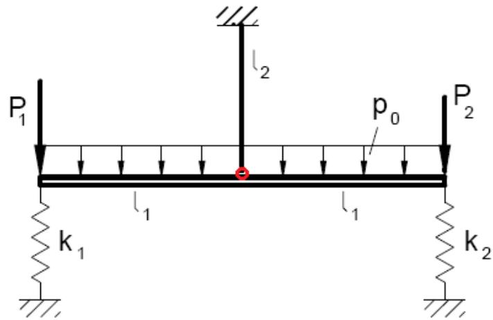
Equivalent forces for constant transversal load:
